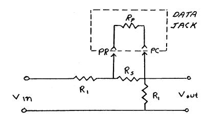
R1 is the source impedance for the input signal Vin, and also the terminating impedance of the load.  $R_{\rm S}$  is a series resistance, on which the computation of the programming resistor Rp is based. The table of values of Rp is derived for  $R_{\rm l}\!=\!600$  ohms;  $R_{\rm S}\!=\!3600$  ohms.
