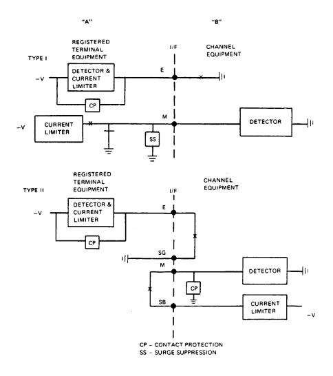
FIGURE 68.3 (e) (i) E&M TYPES I & II SIGNALING
