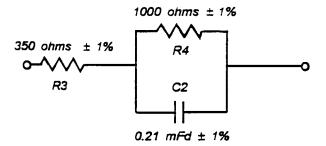
Note: When this alternative termination is used during signal power compliance testing, it replaces R1 (600 ohms) in the loop simulator circuit.
