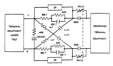
Resistances (Ohms), Capacitances (uF), Tolerances ± 2%.
