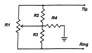
Where:  $R_2 = R_3 = 300$  ohms,  $R_4 = 350$  ohms,  $R_1 = 300$  k ohms, for analog voiceband
