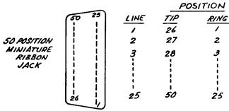
(2) Bridged multiple-line 50-position T/R with make-busy arrangement.
