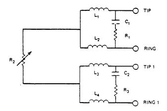
$L_1 = L_2 = L_3 = L_4 > 5H (RESISTANCE = R_{L1}, R_{L2}, R_{L3}, R_{L4})$   $R_1 = R_3 = 600 OHMS, \pm 1\%$  $C_1 = C_2 = 500 \mu FD, \cdot 10\%, + 50\%$
