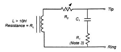
$C_7 = 500 \text{ mFd } -10\% + 50\%$  $R_7 = 600 \text{ ohms } \pm 1\%$  Notes for Figure 68.3(a) apply also to this drawing
