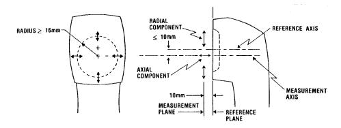
FIG 1 REFERENCE AND MEASUREMENT PLANES AND AXES
