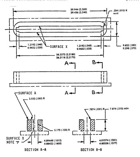
Figure 68.500(e)(2)--50 Position Miniature Ribbon Flug Sizing Guage
