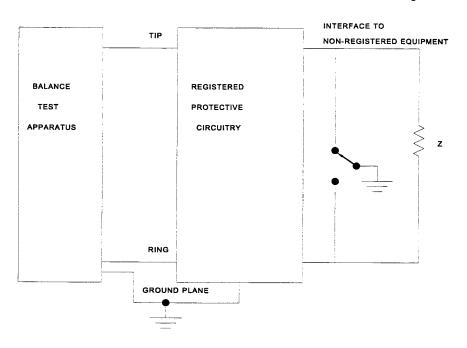
Z - Selected so that the reflected impedance at tip and ring is 600  $\Omega$ , 135  $\Omega$ , or 100  $\Omega$  depending on the service type of EUT
