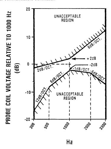
FIG 4A INDUCED VOLTAGE FREQUENCY RESPONSE FOR RECEIVERS WITH AN AXIAL FIELD THAT EXCEEDS -19 dB
