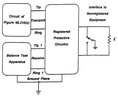
Z Selected so that the reflected impedance at tip 1 and ring 1 is 600  $\Omega$ , 135  $\Omega$ , or 100  $\Omega$  depending on service type of EUT.
