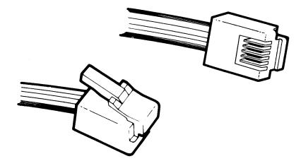
(Note: This plug is depicted equipped with 4 contacts; it may be fabricated with its full 6 contact capability.)
