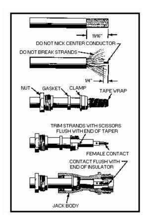
Figure 1-28.—Attaching HN connectors to coaxial cable.
