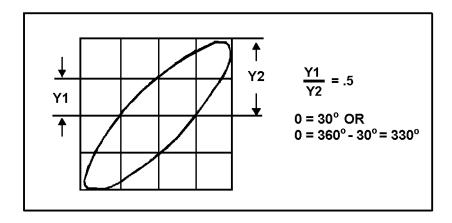
Figure 1-38.—Computation of phase angle.
