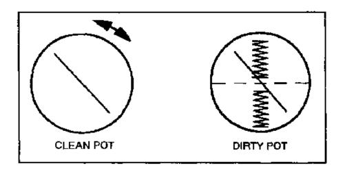
Figure 1-45.—Potentiometer noise check.
