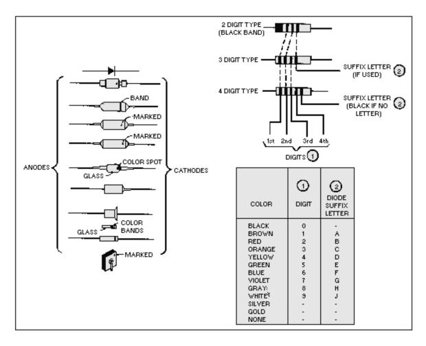
Figure 1-20.—Semiconductor diode markings and color code system.
