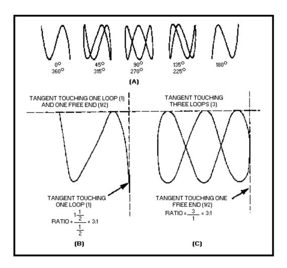
Figure 1-41—3:1 Lissajous patterns and calculation of frequency ratio.
