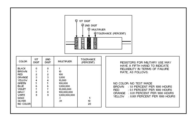
Figure 1-18.—Resistor color code.
