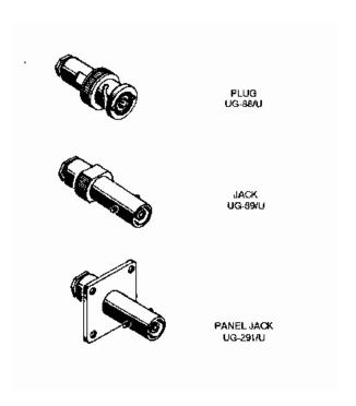
Figure 1-25.—Typical BNC connectors.
