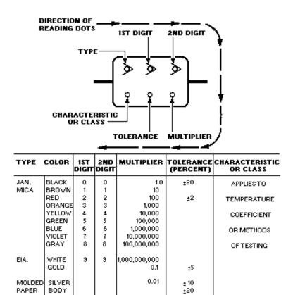
Figure 1-14.—Six-dot color code for mica and molded paper capacitors.
