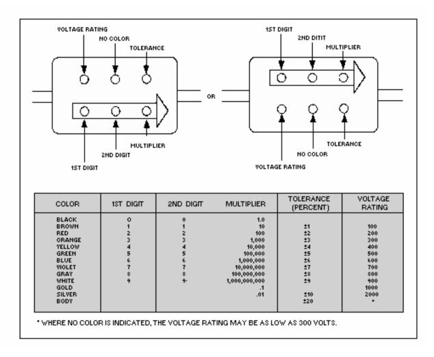
Figure 1-17.—Mica capacitor color code.
