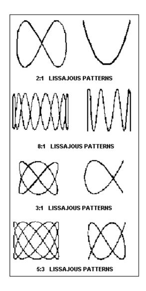
Figure 1-39.—Lissajous patterns of different frequency ratios.
