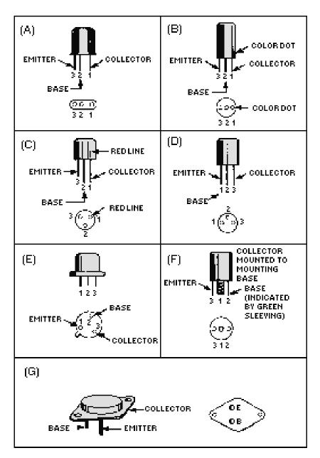
Figure 1-21.—Transistor lead identification and case outline.
