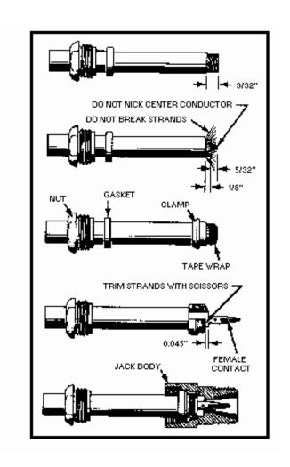
Figure 1-30.—Attaching N connectors to coaxial cable.
