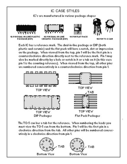
Figure 1-22.—IC identification and pin placement.
