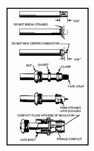
Figure 1-32.—Attaching C connectors to coaxial cable.
