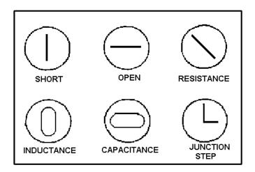
Figure 1-43.—Typical oscilloscope displays for an octopus.
