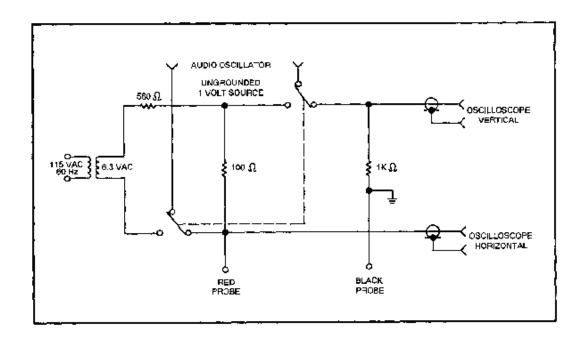
Figure 1-42.—Octopus schematic diagram (typical).
