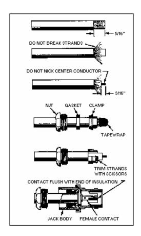
Figure 1-26.—Attaching BNC connectors to coaxial cable.
