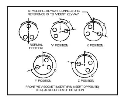
Figure 1-24.—Alternate positions of connector inserts.
