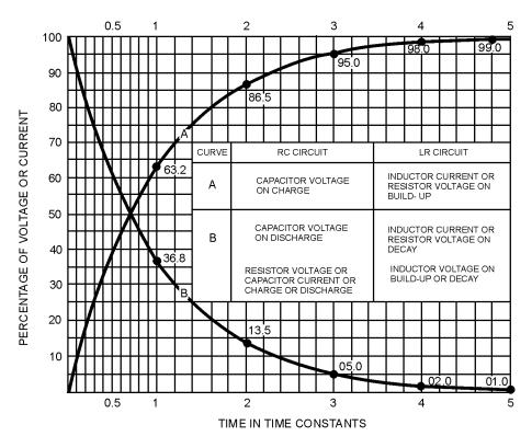
Figure 1-12.—Universal time constant chart for RC and LR circuits.
