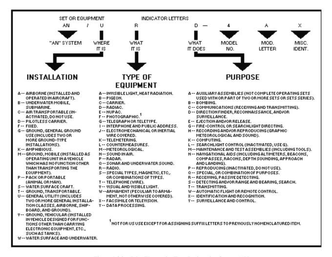
Figure 1-36.—Joint Electronics Type Designation System (AN).
