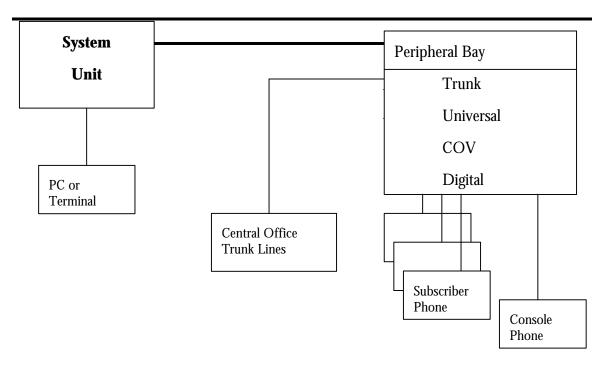
Figure 1. PBX Block Diagram
