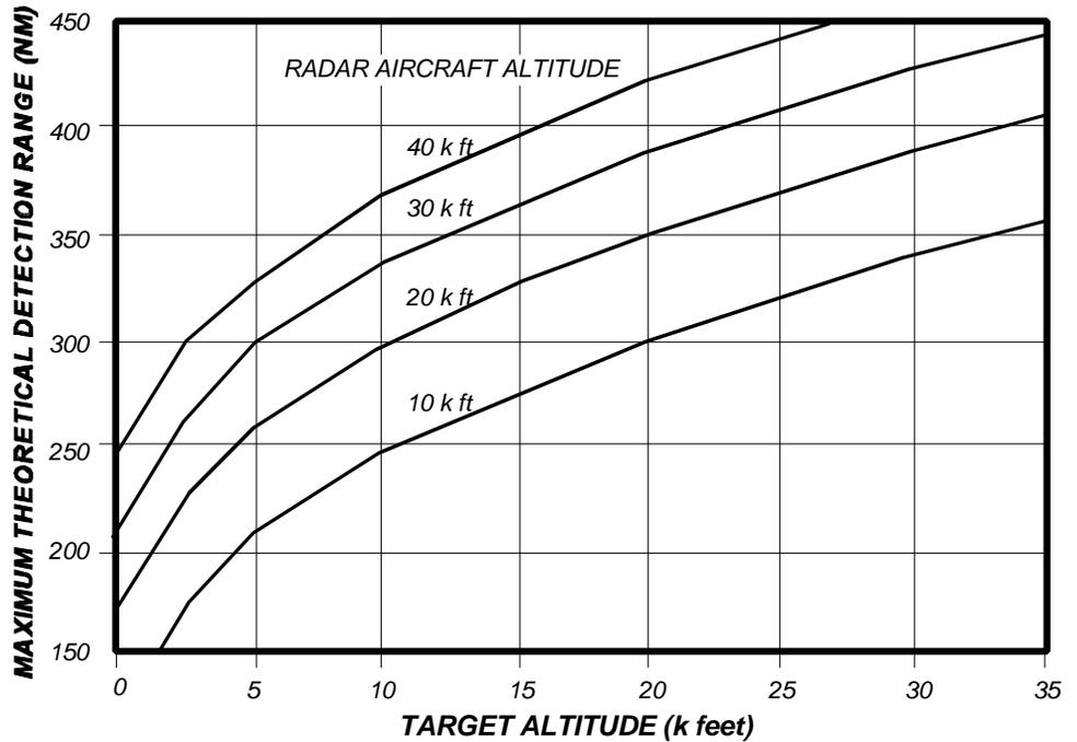
Figure 3. Aircraft Radar vs Aircraft Target Maximum Range
